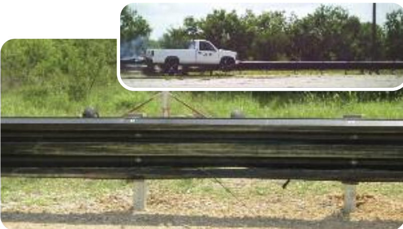
Polyurethane composite guardrail test - ¾ ton pickup truck traveling at 62 Mph: Impact angle 25°
