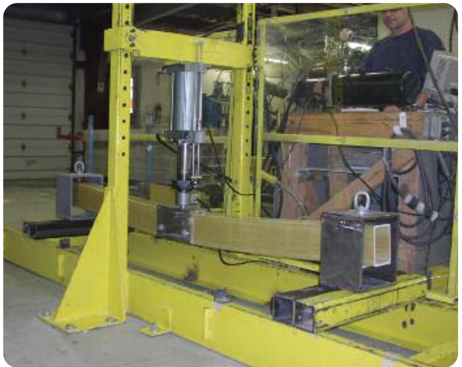
Full section bend test of polyurethane dead end cross arm.
